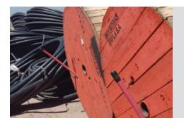
It is made with materials that, in case of fire, do not emit toxic substances or corrosive gases into the environment, thus protecting health and preventing possible damage to electronic equipment.
